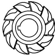
**Heavy-duty shell end mill, with spiral for
