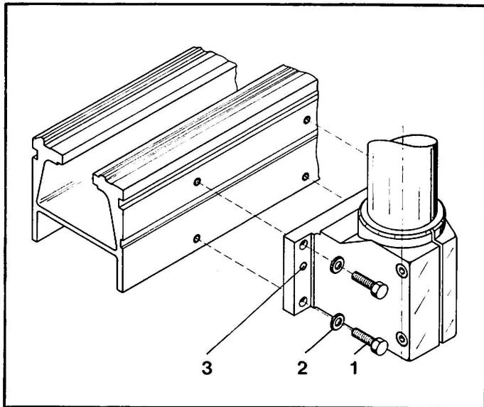
The vertical unit is mounted on the rear of the machine bed with 4 hexagon screws M10x35 ( 1 ) and four washers ( 2 ). The two bolts ( 3 ) must fit into the groove in the machine bed.
