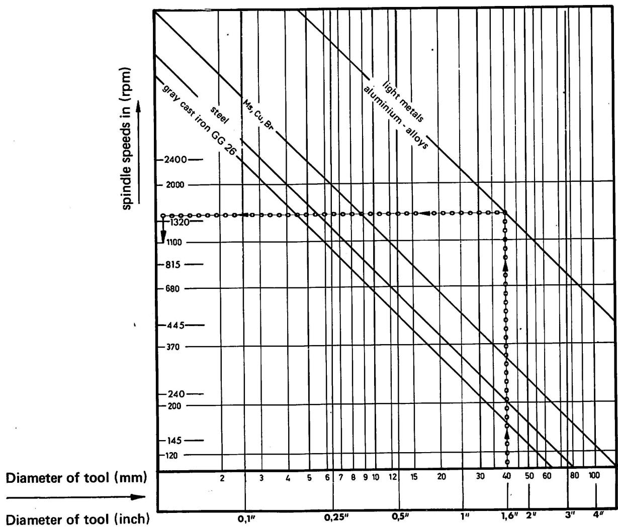
**Example:** Workpiece material: Aluminum alloy
