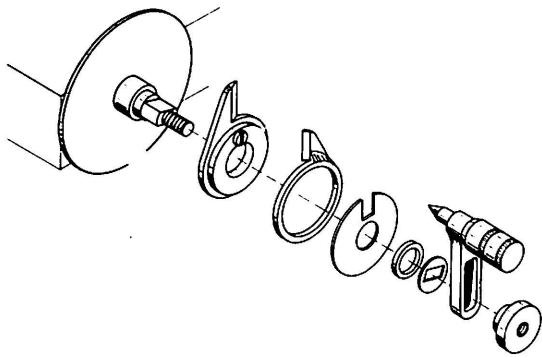
2. In the Indexing Table one sees that at the division 13, 3 full turns plus 3 holes on the 39 plate have to be added. Therefore, the shears are fixed so that they include 4 holes.
