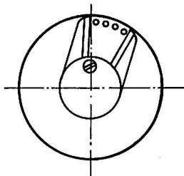
3. The indexing plunger is placed in a hole of the 39 plate (marked black on the drawing) and the left shear arm moved until it touches the pin of the plunger.
